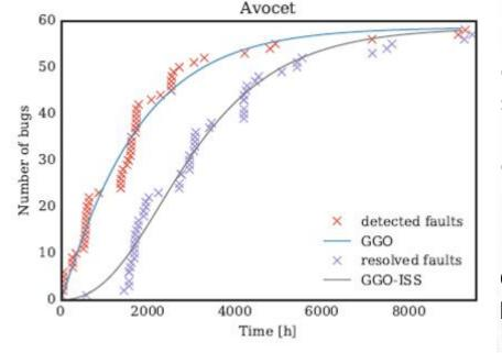
Find best model according to different Goodness of Fit (GoF) such as Mean Square Error, Coefficient of determination, etc.
