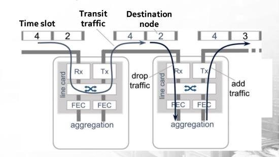
Instantaneous communication without prior path allocation Re-use of reserved but underutilized capacity FEC processing only at end-points
