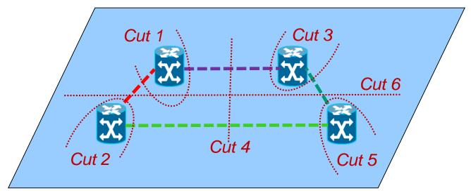
Condition: no physical link shall support all the virtual links in a virtual cutset
